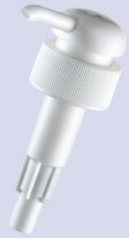
SM25A19 Discharge rate:4.0±0.4ml/T Closure:33/410, 38/410
